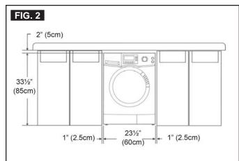
The dimensions shown are for minimal spacing using a custom under-counter installation.
