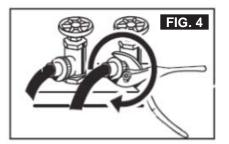
3. Connect the opposite end of the hose to the inlet valve on the backside of the appliance.
