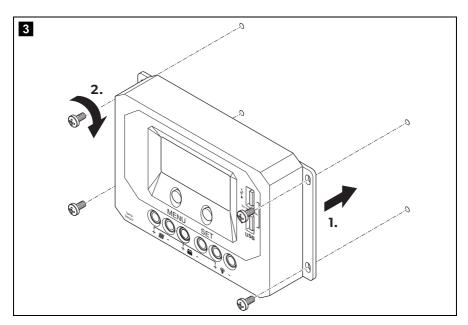
➤ Attach the device with 4 flat-headed screws.
