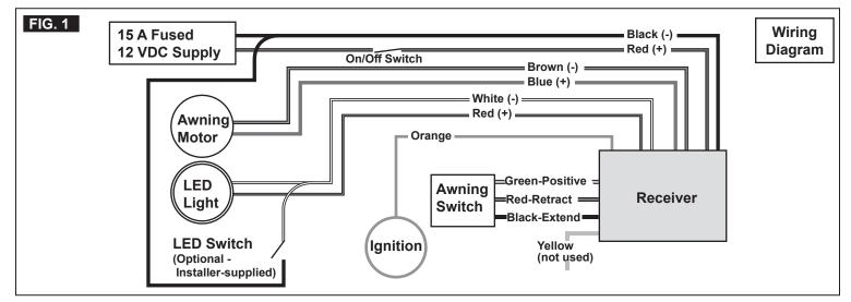
(i) Use the installer-supplied receiver harness connectors, if desired.
