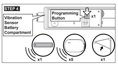
a. Press the vibration sensor programming button. The sensor beeps once, the wireless receiver beeps five times, and the awning jogs.
