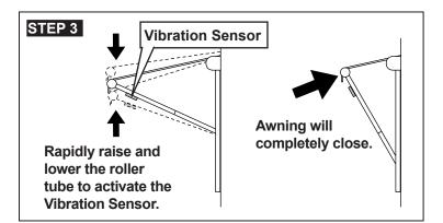
No direct correlation exists between the sensitivity settings on this sensor and true wind speed. The vibration sensor will close the awning any time the motion in the attached hardware arm reaches the pre-set level regardless of the cause of this motion. Wind speed, angle of attack, and the size of the awning are only a few factors that can affect how an awning reacts to environmental conditions.
