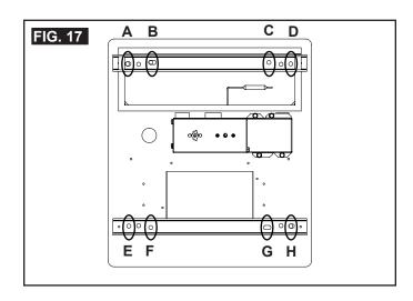
g. **NOTICE** Tighten mounting bolts to correct torque specifications. Overtightening could damage unit's base pan or ceiling template. Not enough torque will allow an inadequate roof seal, and could cause a leak.
