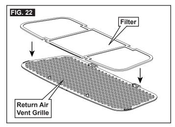
Install return air vent grille into the ADB. Slide return air vent grille tab into slot in ADB and rotate up and snap in place. See (FIG. 23).
