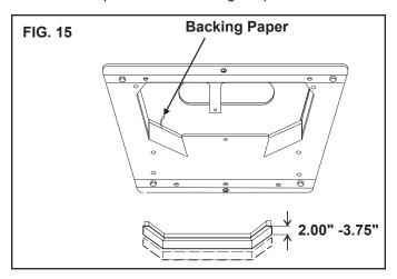
c. Place divider plate up to bottom of the unit base pan firmly. The foam tape on the divider plate must seal to bottom of base pan. See FIG. 16.
