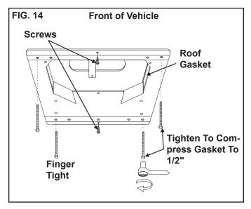
Evenly tighten the four mounting bolts to a torque of 40 to 50 inch pounds. This will compress the roof gasket approximately 1/2". The bolts are self locking so further tightening is not necessary. See FIG. 14.
