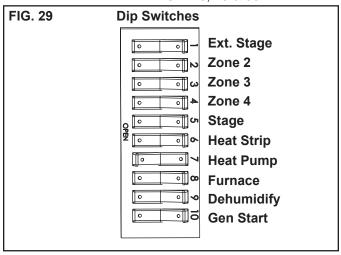
a. Ext. Stage - Ext. Stage is not used on this unit. Leave in the "OFF" position.
