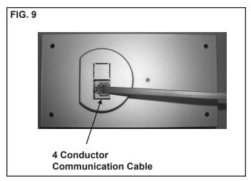
iv. Align the thermostat with the back plate and snap into position.
