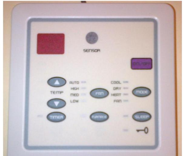
Wall mounted Thermostat control. An AC only model (AC-1361) will not have the furnace pushbutton on the wall pad unit.
