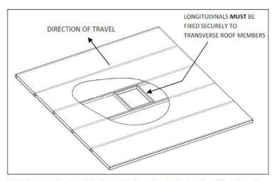
Fig 3: Shows an ideal roof structure with strong longitudinals and a 14' hole boxed
