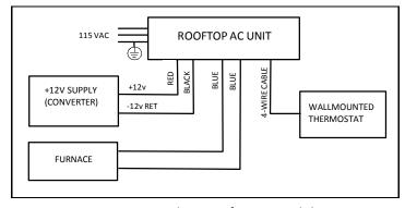
Interconnection diagram for AC models with wall-mounted thermostat
