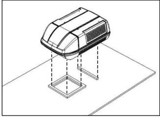
Fig 6- Gently set the unit over the roof gasket..
