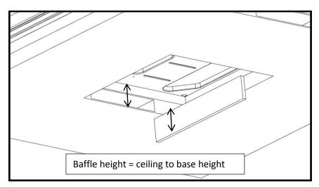
6. Once cut to height insert the baffle into the slot in the plenum deck assembly (3)
