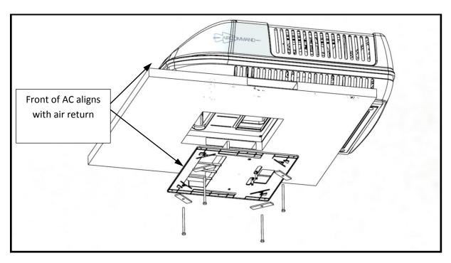
Note: Ensure that the hold down bars (4) are aligned with the recess in the plenum deck before tightening.
