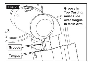
3. **AWARNING** IMPACT OR CRUSH HAZARD. DO **NOT** set Top Casting BEHIND Tongue. Awning roller assembly is **NOT** properly restrained and could become separated. Failure to obey this warning could result in loss of property, serious injury or death.
