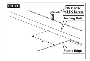
5. Pull to stretch opposite edge of awning fabric approximately 3/4". Then secure with #6 x 7/16" TEK screw through awning rail (approximately 2" from fabric edge).
