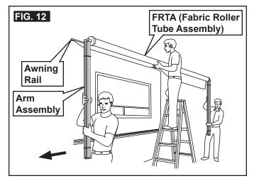
3. While one person guides awning fabric (with awning roller cover, if equipped) into awning rail, carefully move (carry) awning hardware assembly to desired location. See (FIG. 12).
