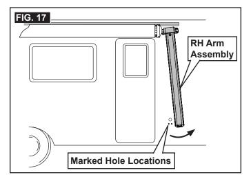
5. Drill 3/16" diameter holes through marked mounting hole locations and into solid structure of RV.
