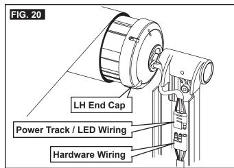
3. LED RAIL LIGHT CONNECTIONS (IF EQUIPPED):
