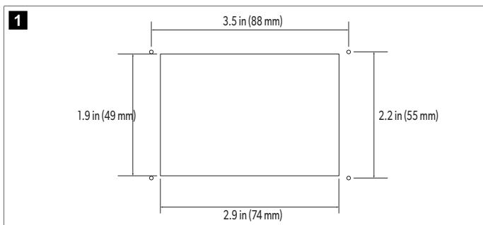
2. Mark the dimensions of the opening and the screw hole locations on the cabin wall.
