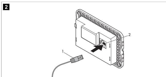
2. Route the other end of the display cable through the wall opening and plug it into the jack on the back of the display.
