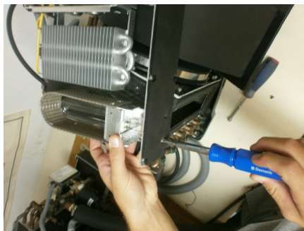
Figure 2: Securing BE to cover panel
