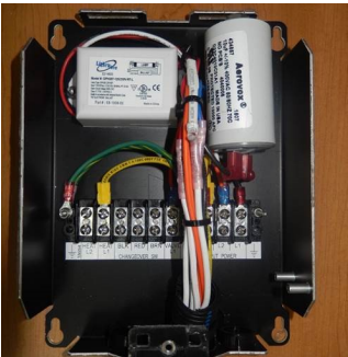
Figure 5: Installation location of ballast in electric box
