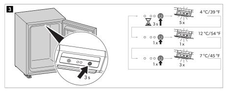
Setting the silent mode (standby) (only for C40S1, C40S2, C40P1, C40P2, C40G1, C40G2, C60S1, C60S2, C60G1, C60G2 with compressor cooling): Fig. 4 on page 9
