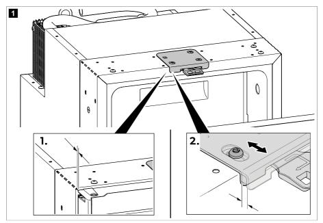
3. If the drawer opens or the opening gap is greater than 5 mm, adjust the door latch position until the opening gap is in the range 2 ... 5 mm ( pig. 1 on page 12, 2.).
