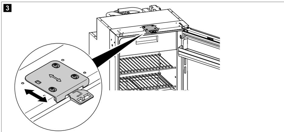
**i** **NOTE** Check whether the adjustable door latch is installed. If necessary, order the adjustable door latch (dometic.com) and replace the fixed door latch with the adjustable door latch.
