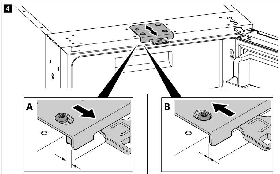
**i** **NOTE** If the door latch is in position **B**, ensure that the door latches properly when closing (see chapter Closing and securing the refrigerator door on page 14).
